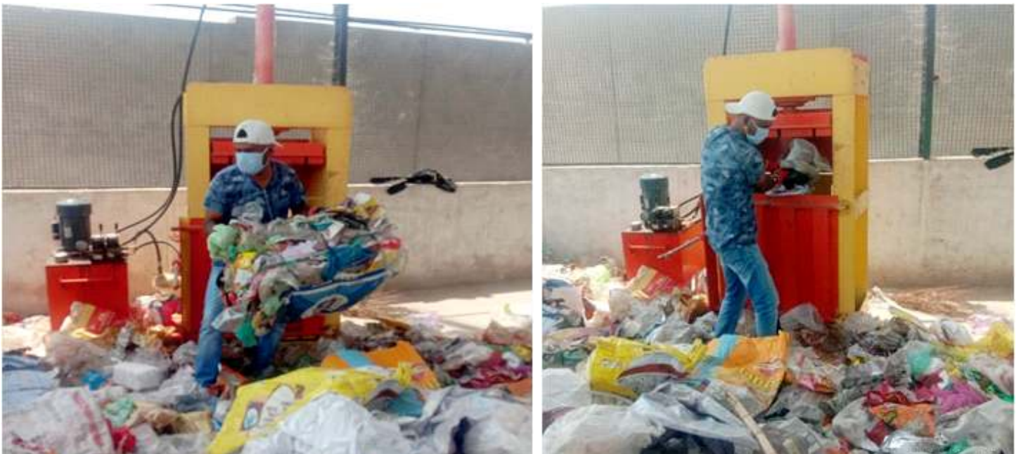
BAILING MACHINE HAS BEEN INSTALLED IN MUNICIPAL COUNCIL UDHAMPUR AT SUI-CHAKAR FOR SCIENTIFIC DISPOSAL OF SEGREGATED PLASTIC WASTE
